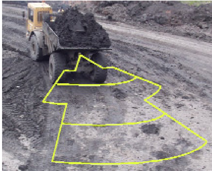
A typical protection zone behind a dumptruck, showing the three stages of warning
